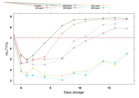
Figure 6.1: Effect of sulphite level on microbial growth in sausages stored in aerobic packaging at  $4^{\circ}C$  (Anon., 2007)<sup>1</sup>
